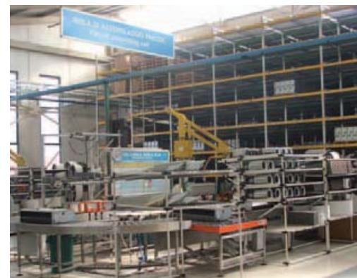
>> The final assembling and packaging cell assembles the cabinets and all components, such as valves, supplementary trays, and the controls.
