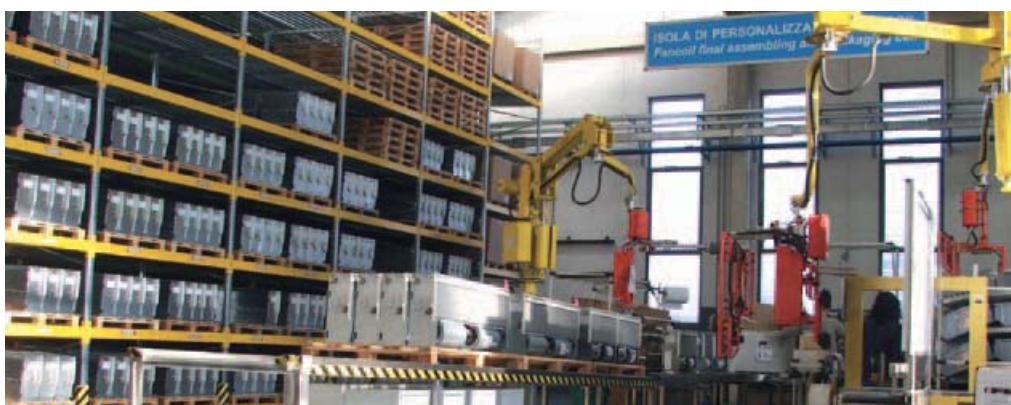
>> Chillers with capacity from 5 to 350 kW are built on the assembly line. The 5 lines total a length of 300 m.
