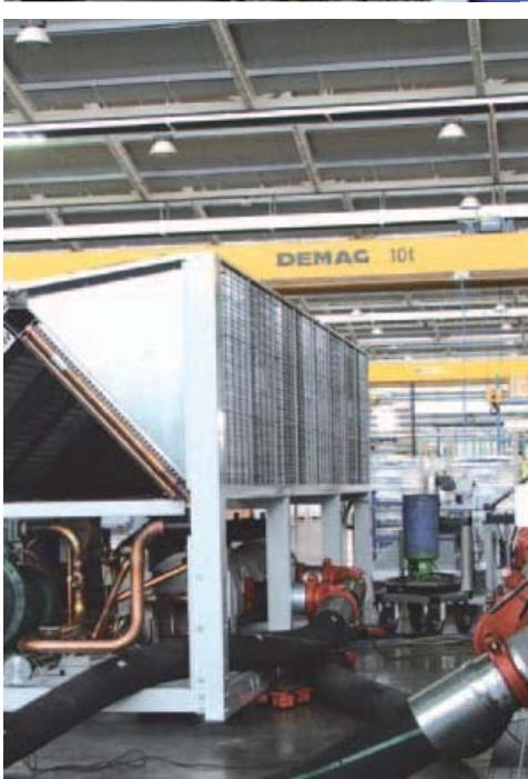
>> For the testing of medium to high capacity chillers (fig. a-b) there are three test chambers which enables units to be tested according to EUROVENT conditions. A very important investment by FERROLI, which offers our customers guarantee that our equipment fully comply the project specification.
